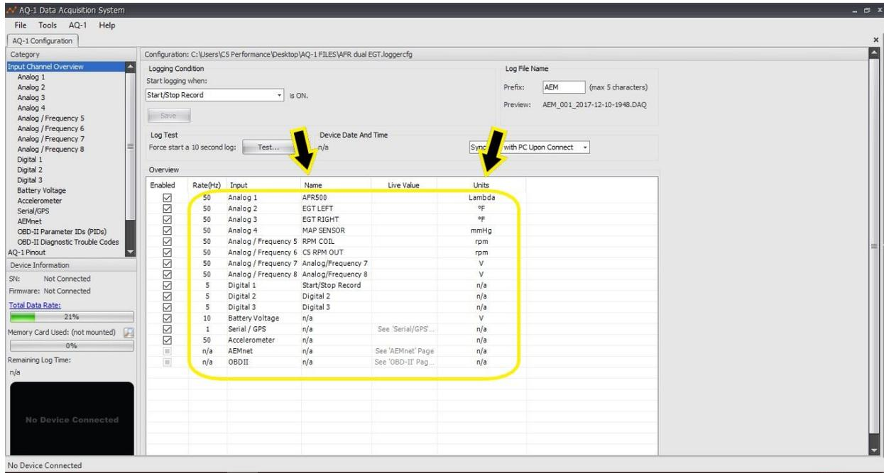
**After you name your inputs the voltage must be calibrated so it accurately records the data. This MUST be done before you start recording. What exactly does that mean? Our AFR500 meter just spews out voltage readings with no real meaning for the logger. By creating a simple chart, the AEM data logging software knows that a certain voltage equates to a certain air-fuel ratio. The formula was provided in the AFR500 meter instructions.**
