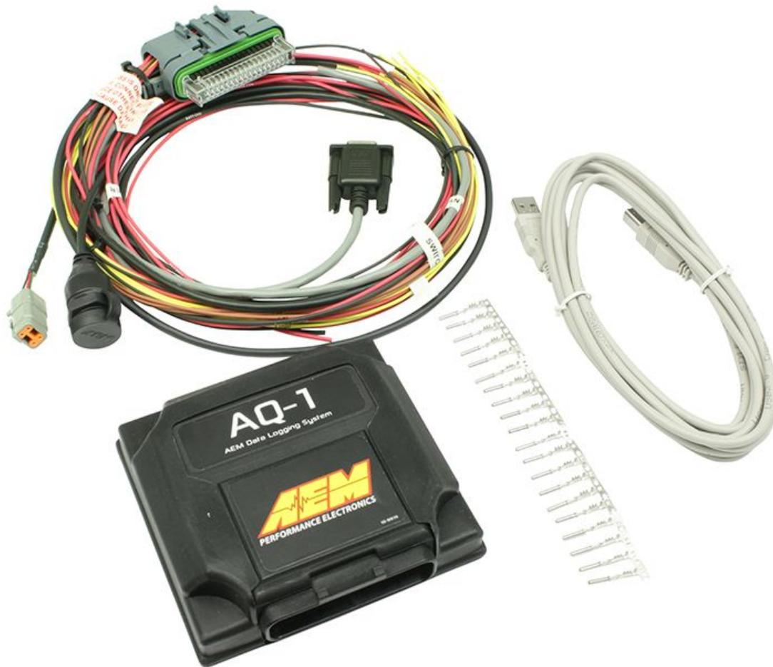
**When shopping for loggers pay attention to refresh rates, measured in Hz. If a logger claims to record at 5 Hz that means it records data five times per second. Some data should be recorded at a faster rate, so we need higher sampling. The AQ-1 can record up to 1,000 Hz on some channels. My AFR oxygen sensor is measured 50 times per second (50 Hz sample rate) and my Garmin GPS is 1 Hz sample rate, which is fine in a 6 mph class.**
