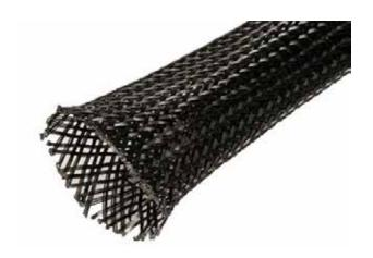
They also offer some that have a slit down them so you can open it up later for repair or adding wires. Most are rated to 500 degrees F heat resistance and the price is reasonable. Sizes range from 1/4" up to well over an inch diameter.
