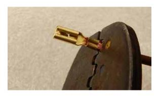
The insulator should be just sticking past the first crimp. You can solder the connector afterward but never allow the solder to creep past the first crimp or failure is likely.
