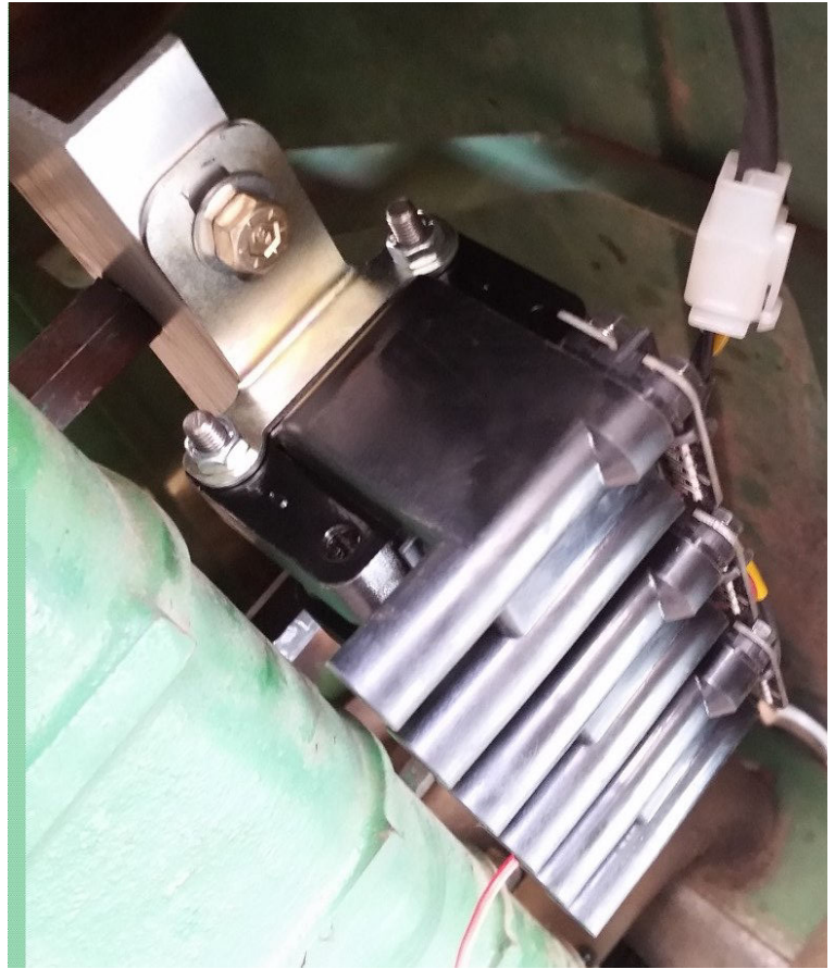
Sample pictures showing coil mounting.
