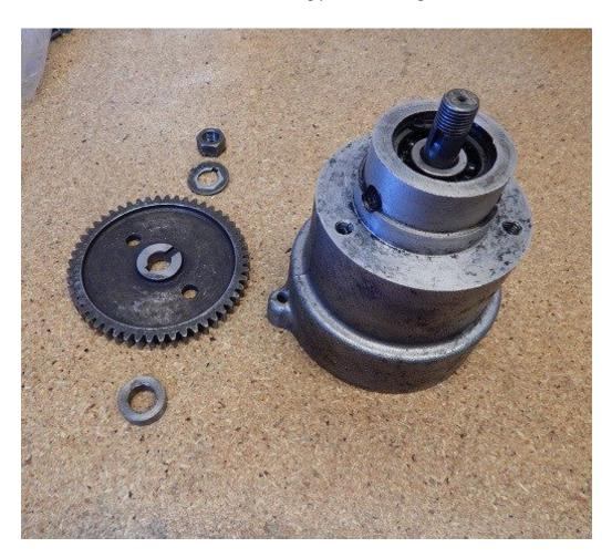
**Step 2:**Install new timing shaft using supplied parts.
