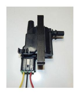
The newest MC (micro coil) has a different wiring harness than other motorcycle coils.
