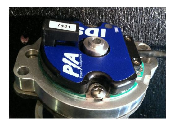
Once the stock ignition is removed, install the aluminum adapter plate using the stock screw, and then install the new ignition module. For timing purposes you may have to install the cap screws while the timing is set.
