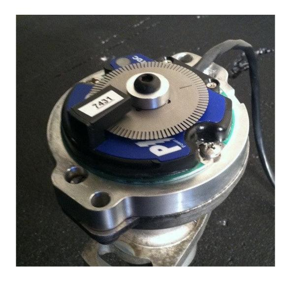
This is what your assembled ignition should look like. The top cap can be re-installed using the new longer screws provided.
