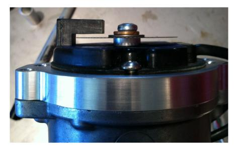
The cap is not the style your kit has but please observe the spacing of the encoder. There should be space above and below the encoder disc.
