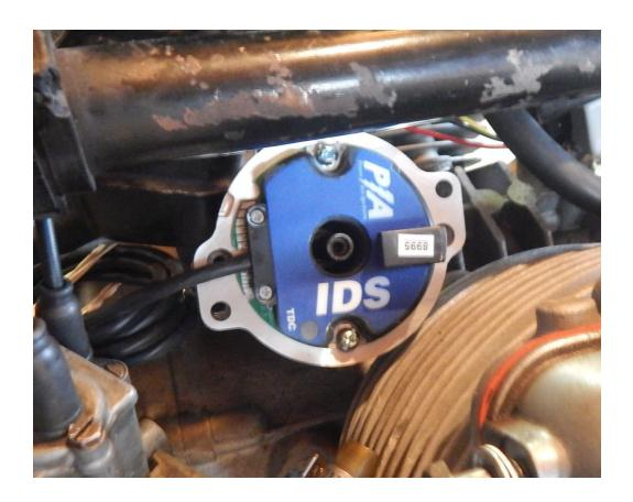
Install your aluminum adapter plate using the same screws you removed with the contact points plate. Insert the ignition module on top and secure using the screws provided in the kit.
