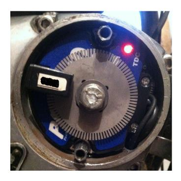
A small red LED light will come on. At this point carefully tighten the encoder disc to the distributor post.
