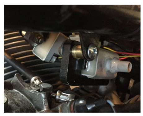
Coils can be mounted on frame in several areas or clamped on using rubber coated plumbing clamps.
