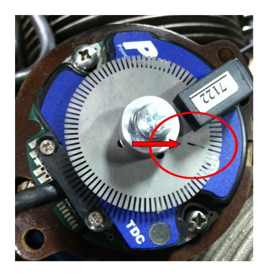
Match the encoder disc to your engine to set TDC on the ignition module:
