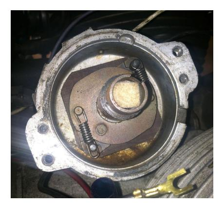
Remove the advancer weights and springs. All that should be left is the shaft and base plate.
