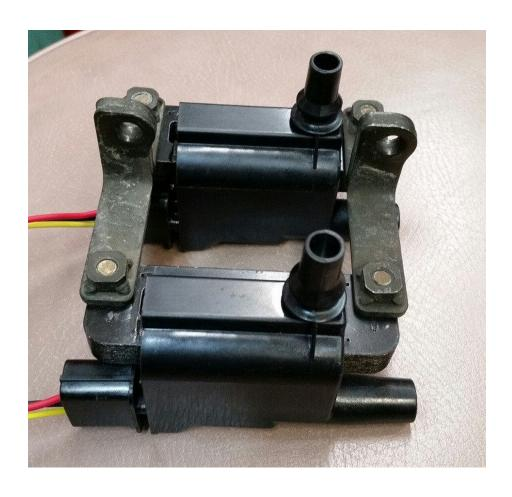
This shows how the MC2 coils fit the stock GL1100 with no additional hardware.
