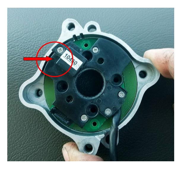
Set timing. The LED light is located next to the reader. When this slot passes under the reader, the LED light will come on and your timing will be set.
