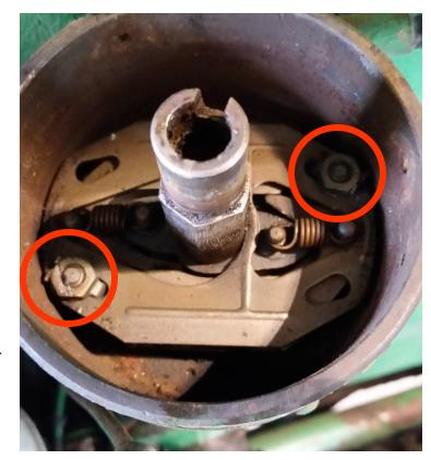
This is what it looks like with all parts removed. Now you will install the adapters and test fit height of encoder disc.
