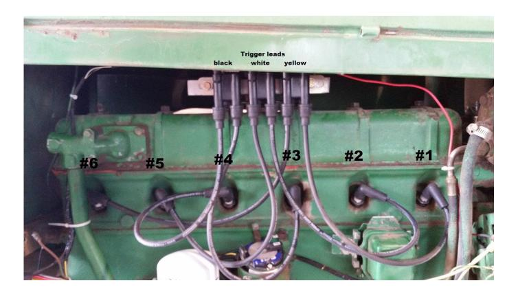
This is the firing order used on Oliver 770 with inline 6 cylinder (as example)
