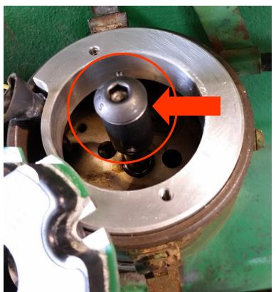
This picture shows correct disc height. We have designed the center piece so that if you slide it over the distributor shaft with the center screw installed, it should be at the correct height.
