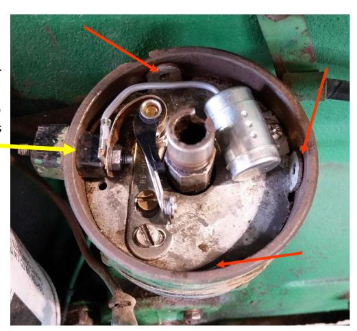
Once timing plate is removed the timing fly weights also need to be removed. Using a small flat blade screw driver or punch, flatten the lock tabs and remove these nuts.
