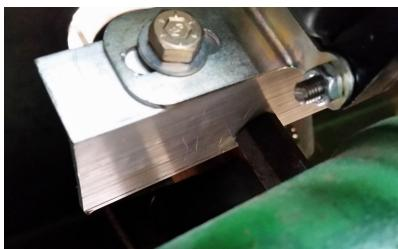
These photos show the coil towers facing down. We recommend when possible the towers face horizontal or upward to avoid wires slowly sliding out of the coil.
