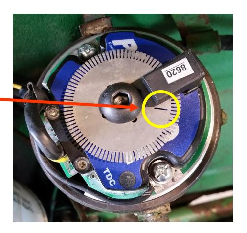
Route wires up and over circuit board so if you need to re-program in the future the wires do not get in the way.
