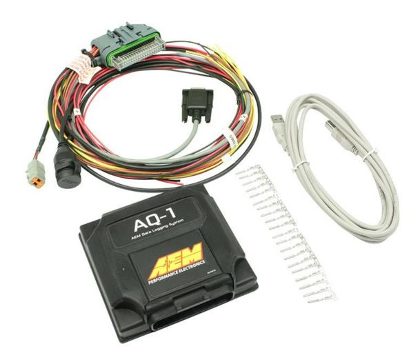
When shopping for loggers pay attention to refresh rates, measured in Hz. If a logger claims to record at 5 Hz that means it records data five times per second. Some data should to be recorded at a faster rate, so we need higher sampling. The AQ-1 can record up to 1,000 Hz on some channels. My AFR oxygen sensor is measured 50 times per second (50 Hz sample rate) and my Garmin GPS is 1 Hz sample rate, which is fine in a 6 mph class.
