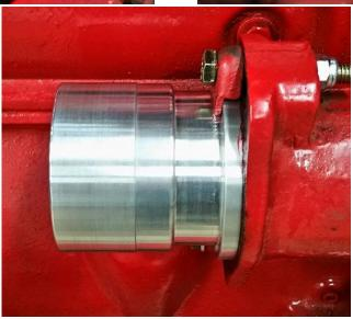
Install encoder disc and set timing.
