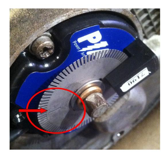
You can clearly see the small slot in the encoder wheel. When this slot passes under the reader, the LED light will come on and your timing will be set.
