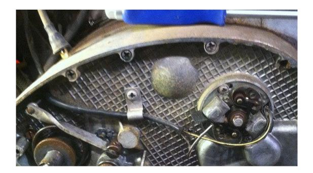
Before setting the timing and tightening the encoder, you must first set the engine at Top Dead Center (TDC) or the ignition will not fire at the correct time.
