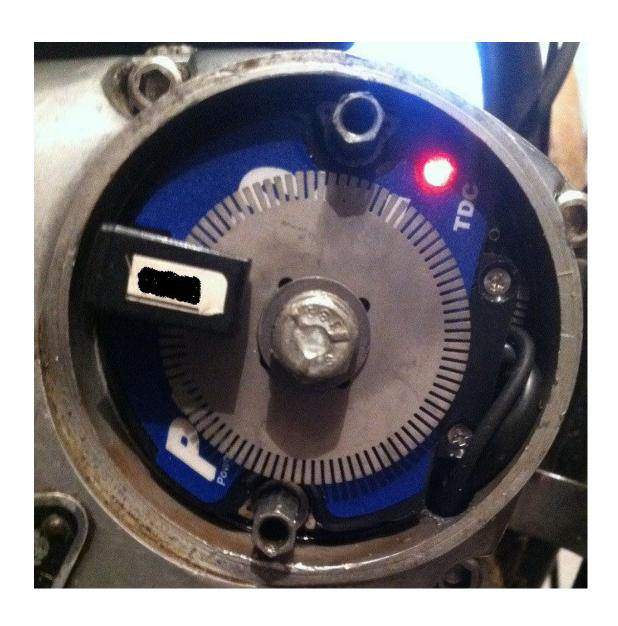
We notice improved starting effort and often no longer need to "feed it throttle" when starting. Customers typically notice faster warm ups due to the multi-spark function of the ignition coil. If you regularly ride in wet weather apply a small amount of silicone where the wires exit the points area. The encoder is stainless steel and shouldn't corrode under normal riding conditions.
