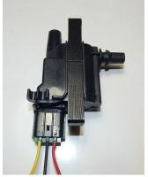
Dual Tower coils are designed to fire two cylinders at once. This is called "wasted spark" because it fires each cylinder regardless of which stroke it is on. We use a pair of these on dual plug cylinder heads.
