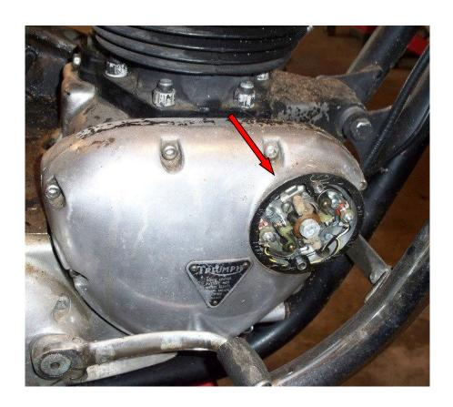
Preparation and installation of new ignition. On Triumphs, It is recommended to chamfer the factory hole where the wiring exits the points area. Use a small file or die grinder to carefully round the hole. This will make it much easier to pull the new wires without damaging them. A pinched wire can cause ignition failure or even a fire.
